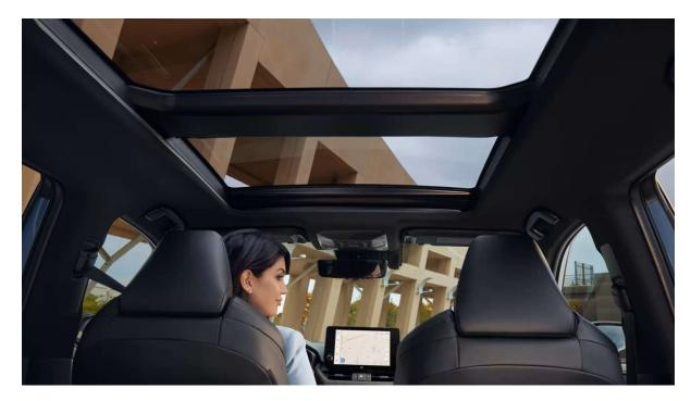
66. Upon information and belief, Toyota makes its panoramic roofs out of tempered glass, also called a safety glass as when it breaks it separates into small pieces. Tempered or safety glass is made by shaping and cutting a piece of annealed glass that is then heated and rapidly cooled. This tempering process creates an outer layer of compression that is shrinkwrapped around the middle of the glass, which is constantly pressing outwards, making the final
